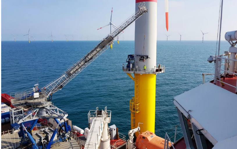
Fig 2 – Ampelmann motion compensated gangway system
