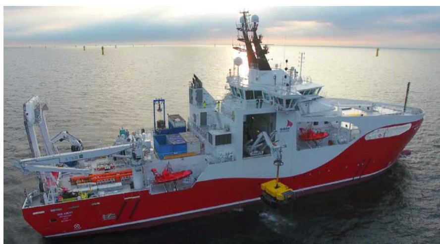
Fig 4 – trenching vehicle being deployed from vessel.
