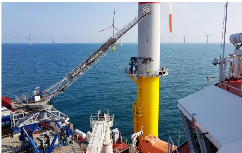
Fig 2 – Ampelmann motion compensated gangway system
