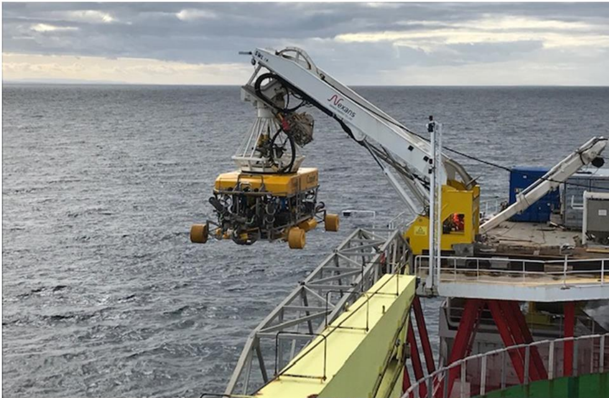
Fig 3 – Capjet trenching tool deployment.
