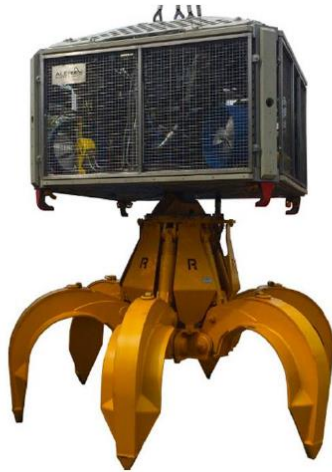
Fig 2 – ROV with integrated grab tool.
