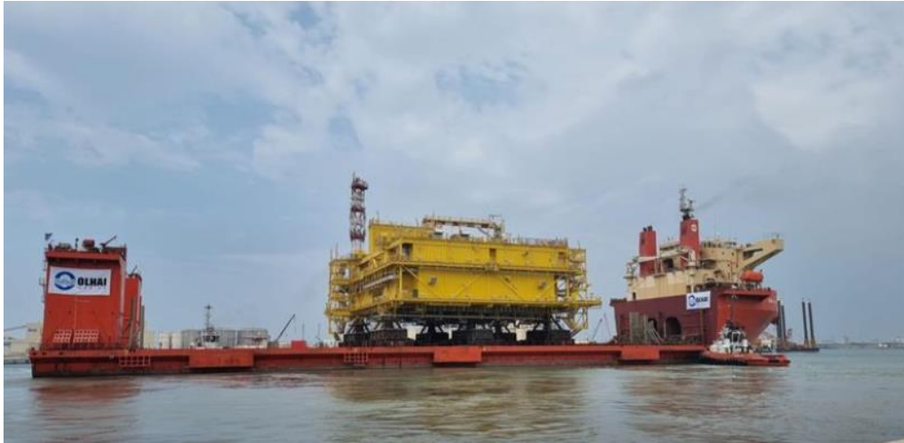
Fig 2 – OSP topside structure aboard Heavy Transport Vessel Sun Rise.
