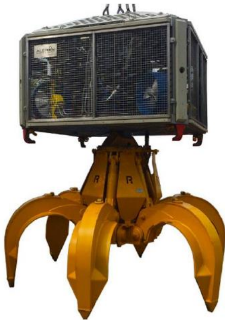
Fig 2 – ROV with integrated grab tool.
